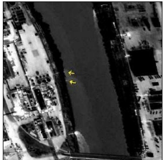
Figure 18: Four discharges to the river appear as white plumes. The two discharges highlighted with arrows were unknown discharges. (Source: http://www.excel.net/~jdh/products1.html )
