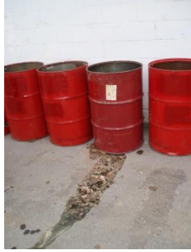
High Severity Chemicals Management – Uncovered, unlabeled leaking barrels
