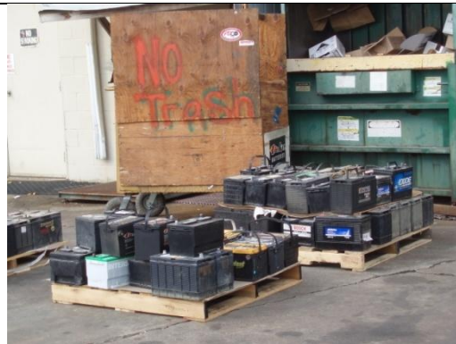
Moderate Severity Chemicals Management – Batteries outside without cover, on pallets
